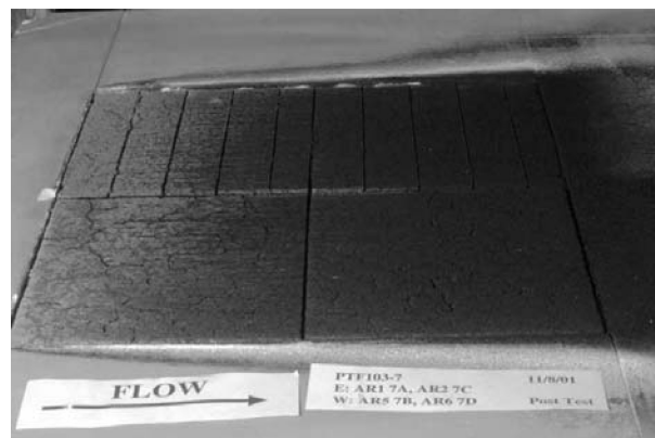
Fig. 10c Posttest photo of ARA Hyperlite materials from test at 17 W/cm 2 .
