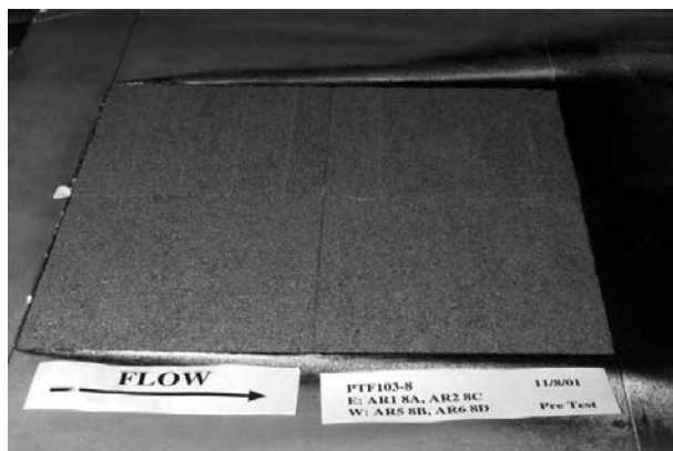
Fig. 10a Pretest photo of ARA Hyperlite silicones with a mixture of low-density fillers.
